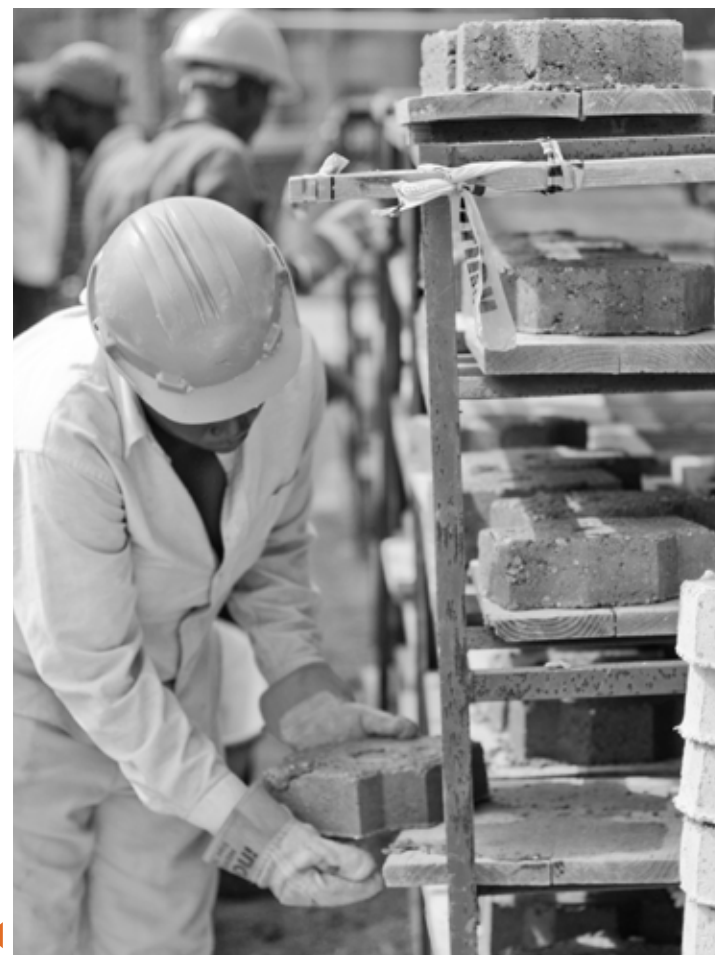
Workers making paving stones out of recycled debris. Demolition and Debris removal Project
